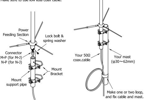
Note: For long-term use, water-proofing with glue, self-fusing tape, and/or vinyl tape is highly recommended.
