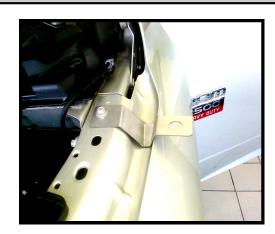
Please Read: Always check for continuity between the bracket and chassis ground. If there is a problem with grounding, place the provided star washer between the bracket and the fender.
