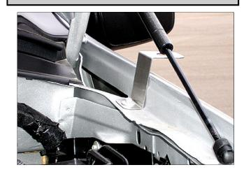
Please Read: Always check for continuity between the bracket and chassis ground. If there is a problem with grounding, place the provided star washer between the bracket and the fender.
