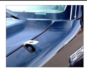
Please Read: Always check for continuity between the bracket and chassis ground. If there is a problem with grounding, place the provided star washer between the bracket and the fender.
