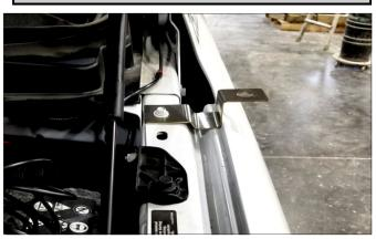
Please Read: Always check for continuity between the bracket and chassis ground. If there is a problem with grounding, place the provided star washer between the bracket and the fender.
