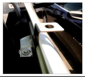
Please Read: Always check for continuity between the bracket and chassis ground. If there is a problem with grounding, place the provided star washer between the bracket and the fender.
